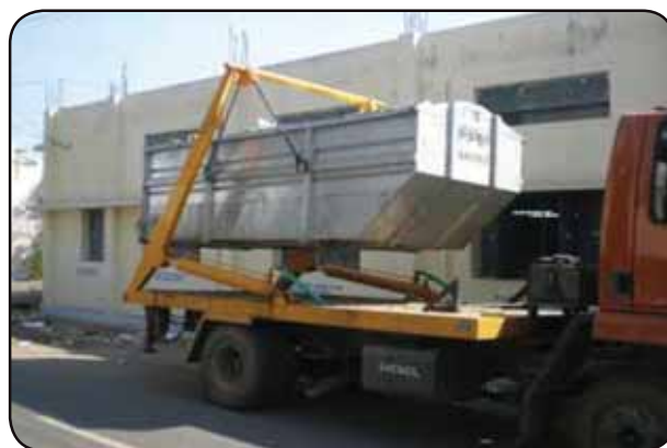
Dumper Placer in Operation
