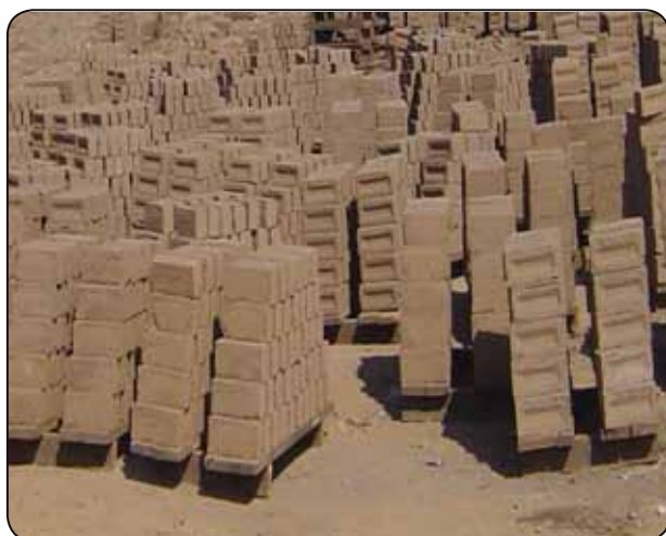
Bricks manufactured through inert material
