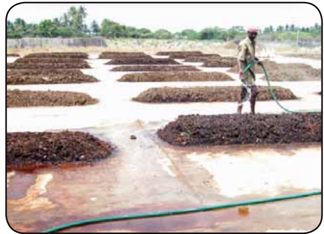
Windrows Moisturing - Extra watering leads to leachate generation
